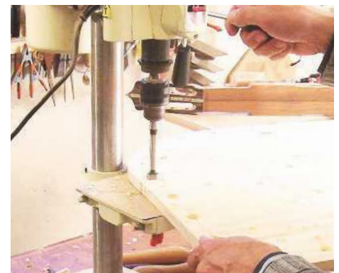
▲ Pic.6 The drill press comes in handy when cutting a series of holes
